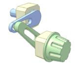
The video shows case when the green link rotates 90 deg., the blue rotates 180 deg.
