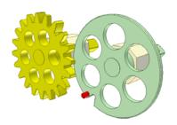
gear. The mutilated tooth between them is in front of the driver. At the end of the dwell period, the red pin contacts the mutilated tooth and turns the driven gear around one circular pitch. Then the full-width tooth engages the tooth groove and the driven gear moves around one more pitch. The dwell period starts again and the cycle is repeated. Totally in one revolution of the driver, the driven gear turns two circular pitches.
